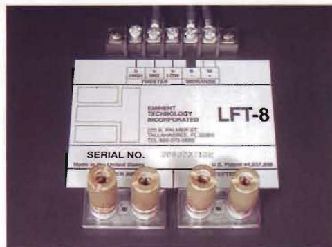
The bi-wire rear terminal panel also carries High, Mid and Low tweeter settings.
